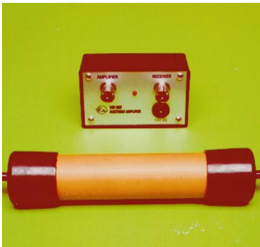
The amplifier itself is housed in a length of 32mm OD PVC tubing, with close-fitting end caps (front). The matching power feed unit is in the small utility box at rear, which connects at the foot of the co-axial download.
